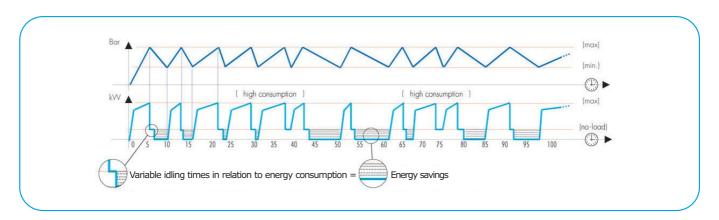
When there is no or very little need for air, the compressor goes into idle mode as soon as it reaches maximum pressure. Energy savings are obtained by stopping the compressor after the shortest idling time possible, which means that the compressor:
